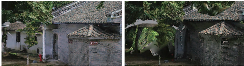
Comparison of the model of the part of Huang Xing's former residence behind the house obscured by trees (The left is the result of the 3D model after fusing drone and Hi-Target vRTK data The right is the result of the 3D model from UAV tilt photography)
